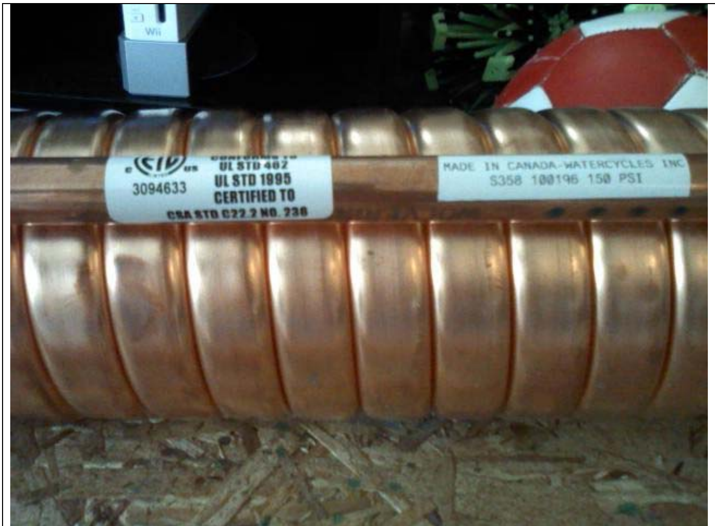
Fig. 1 Photo showing ETL labels on one of 3 substandard Watercycles' GFX's with no incise mark o coil.
