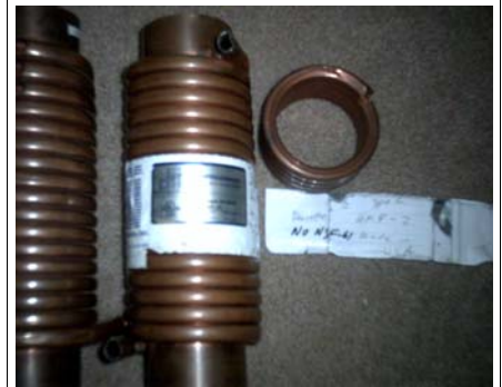
Fig. 3 Doucette GFX/PowerPipe & Coil Section. The latter has no ASTM B88 or ANSI/NSF-61 mark; only the following incise mark: " 1/2" Type L HMP-Z MADE IN USA ".
