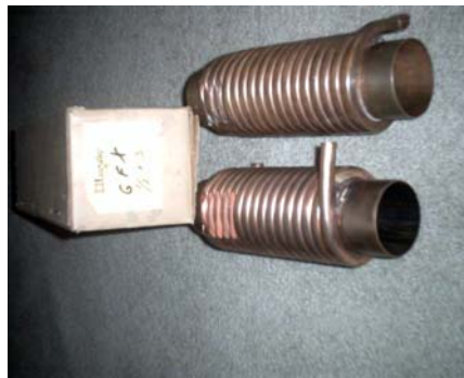
Fig. 2 Two Vaughn G3-12's before coil Removed from lower unit.
