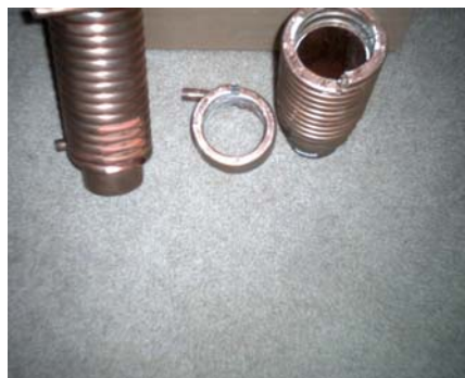
Fig. 4(b) Cut & intact Vaughn G3-12's. No continuous yellow stripe on 3" central DWV drainpipe.
