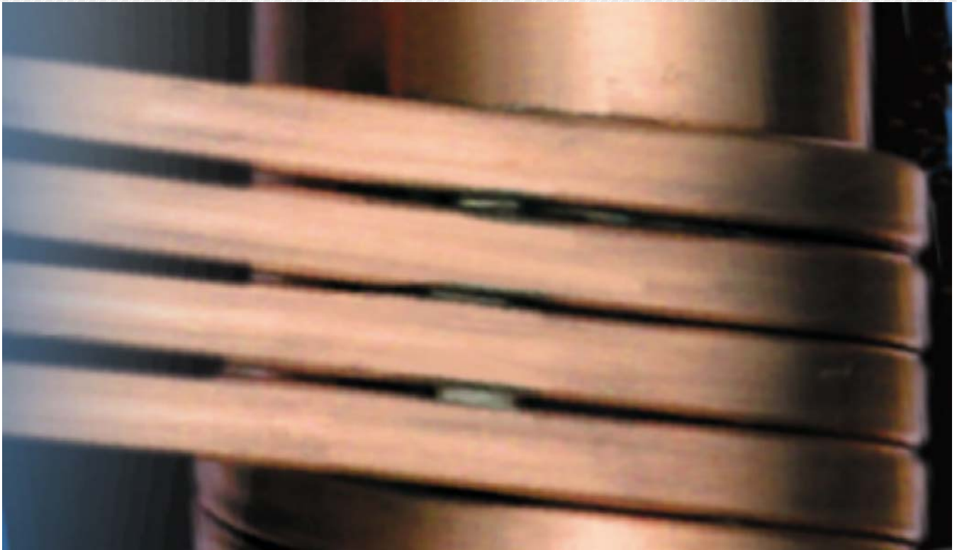
Fig. 1 Power-Pipe end enlargement from Fig 2 below shows coils are soldered directly to drainpipe. This does not meet double-wall venting requirement of UL File SA8583 (7/92) ; the original GFX safety certification licensed to Doucette Insustries then pirated by Renewability.
